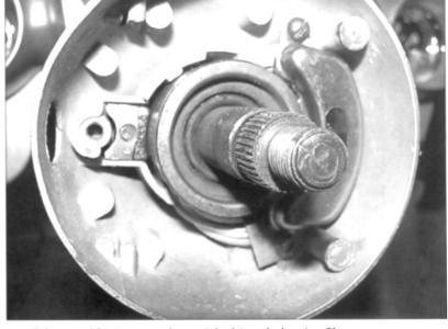
Install the coated friction nut and screw it back into the housing. Place it where you need it, tighten it and you won't need to tighten it again. The increased friction of the now attached rubber firmly grips the smooth painted surface so that even small amounts of pressure will hold it firm. Reassemble the canceling mechanism, and replace the steering wheel and horn button and you're ready to enjoy many miles of Corvette driving with signal lamps that cancel again!
