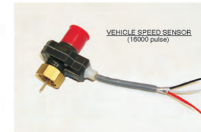
Typical 3 wire Autometer 5291 VSS connection
